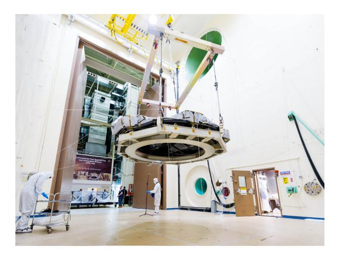
Technicians prepare for acoustic testing at NASA's Goddard Space Flight Center in Greenbelt, Maryland. During testing, the Deployable Aperture Cover for NASA's Nancy Grace Roman Space Telescope was suspended in the air and exposed to 138 decibels for one full minute to simulate launch's intense noise. Credit: NASA/Chris Gunn
