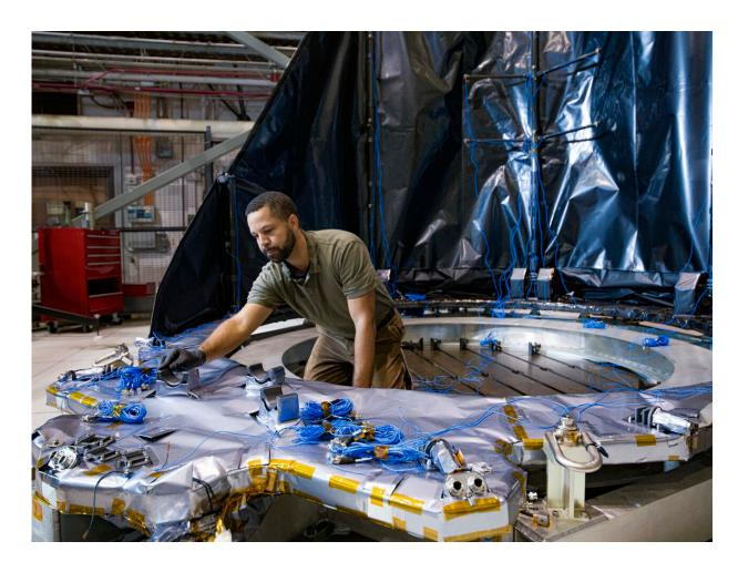
Brian Simpson, product design lead at NASA's Goddard Space Flight Center, adjusts sensors on the Deployable Aperture Cover for NASA's Nancy Grace Roman Space Telescope. The sensors will collect data on the DAC's response to testing. Credit: NASA/Chris Gunn
