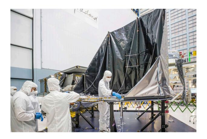
After a successful test deployment at NASA's Goddard Space Flight Center in Greenbelt, Maryland, clean room technicians inspect the Deployable Aperture Cover for NASA's Nancy Grace Roman Space Telescope. Credit: NASA/Chris Gunn
