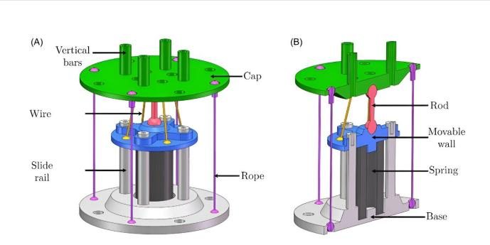
Three-dimensional virtual prototype model of the proposed negative-stiffness device: (A) full view and (B) cross-sectional view. Credit: *International Journal of Mechanical System Dynamics* (2024). DOI: 10.1002/msd2.12118
