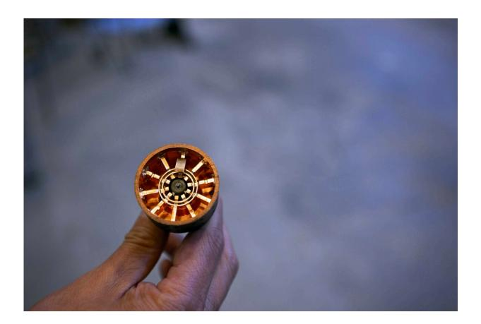
Jefferson Lab Senior SRF Accelerator Physicist Haipeng Wang displays the resonant chambers within the core of a cavity magnetron. Credit: Jefferson Lab photo/Aileen Devlin
