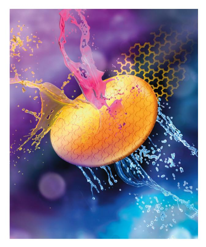
The image illustrates the tunable wettability of a dual-faced covalent organic framework (COF) membrane synthesized viamicrowave-mediated interfacial polymerization. The membrane showcases superhydrophilic and near-
