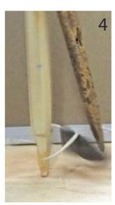
A high-speed photo sequence during a test after an 11.34 kg weight was dropped from 35 cm shows various moments as the stone point recedes into and splinters the pike shaft. Researchers said the way the stone point could have pierced animal flesh and the wood-and-bone shaft opened up suggests that the spear as a system functioned similar to a hollow-point bullet. Credit: Scott Byram
