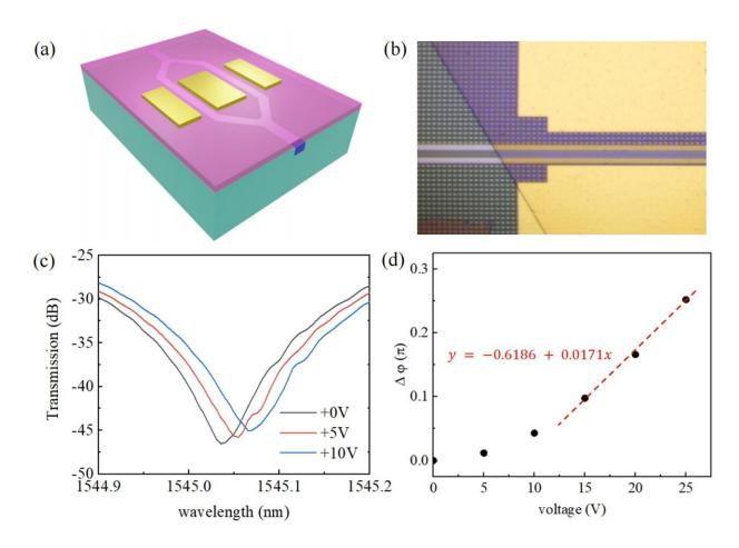
(a) Simulated schematic of the MZI device; (b) Optical micrograph of the MZI device at the waveguide; (c) Measured transmitted light intensity spectra at selected voltages of +0 V, +5 V and +10 V; (d) The curve is calculated with respect to different voltages, with the red line being the tangential of the curve. Credit: *Light: Advanced Manufacturing* (2024). DOI: 10.37188/lam.2024.031
