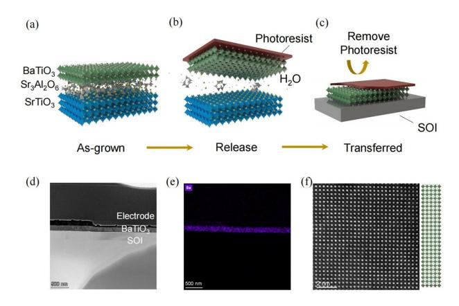
(a)-(c) Schematics of single crystal BTO peeling-off and transfer process from strontium titanate (STO) to the SOI substrate; (d) Cross-sectional transmission electron microscopy (TEM) image of a contact/BTO/SOI heterostructure; (e) Energy dispersive X-ray spectroscopy (EDS) element mapping of Ba element; (f) Atomic resolution scanning transmission electron microscopy (STEM) image of BTO layer. Credit: *Light: Advanced Manufacturing* (2024). DOI: 10.37188/lam.2024.031
