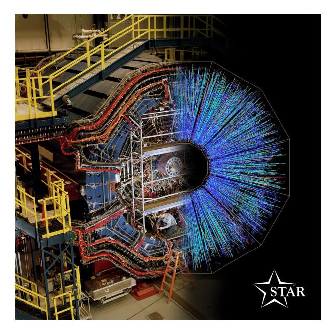
Composite image of the STAR detector and an example of particle tracks it detects emerging from a gold-gold collision at the Relativistic Heavy Ion Collider (RHIC) at Brookhaven National Laboratory. Credit: Joe Rubino and Jen Abramowitz/Brookhaven National Laboratory
