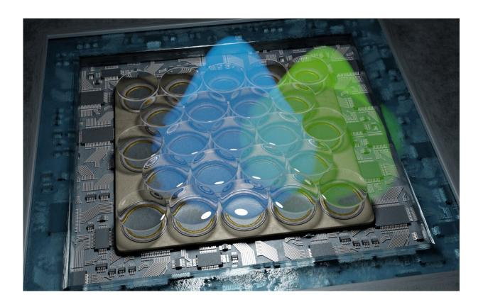
Representation of the highly sensitive detector that is part of the newly developed fluorescence microscope. It consists of 23 individual detectors, enabling the resolution to be doubled. Credit: Alexey Chizhik, Göttingen University
