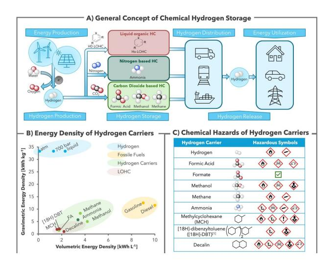
The principal concept of chemical hydrogen storage considering energy density and chemical hazards of hydrogen carriers. Credit: *Nature Communications* (2024). DOI: 10.1038/s41467-024-51658-2
