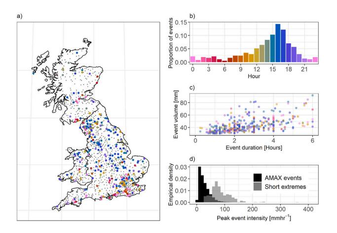
a) Geographical and b) hourly distributions of UK rainfall events with duration under 6-hrs that match or exceed an intensity of 30 mm h–1 between 2000 and 2020, c) scatterplot of event duration and volume, and d) Comparison of the peak event intensity [mm hr–1] empirical distributions for a large ( $\sim$ 72,000) sample of annual maximum events (of any duration) and for short extremes (
