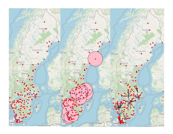
Step-by-step development of hub networks across Swedish MWWTPs based on criteria in Section 2.2.3. The left panel indicates plants meeting the hub criteria in blue, with other examined MWWTPs shown in red. The middle panel displays groups of plants within a 100 km buffer zone around the selected hubs. The right panel illustrates the final hubs and the plants connected to them. Credit:
