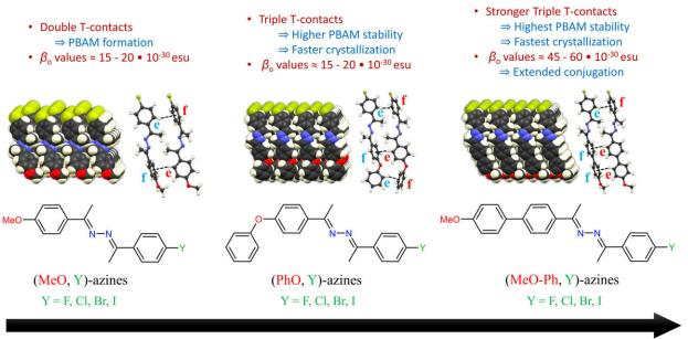
Increasing crystal lattice stabilization and NLO performance
