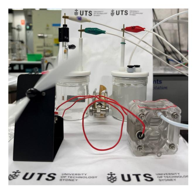
The reaction cell for simultaneous hydrogen production and ammonia oxidation. Credit: *Advanced Energy Materials* (2024). DOI: 10.1002/aenm.202401675
