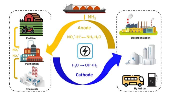
Electrolysis of ammonia aqueous solution produces nitrite and nitrate on the NiOOH-Ni anode, and green hydrogen on the Ni<sub>2</sub>P-Ni cathode. This presents advantages over the currently used thermal ammonia cracking due to the simultaneous formation of hydrogen as an energy carrier and nitrite and nitrate as valuable chemicals under ambient conditions. Credit: *Advanced Energy Materials* (2024). DOI: 10.1002/aenm.202401675
