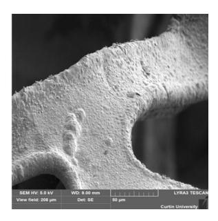
Scanning electron micrograph of the catalyst, NiOOH-Ni, developed in this study. Credit: *Advanced Energy Materials* (2024). DOI: 10.1002/aenm.202401675
