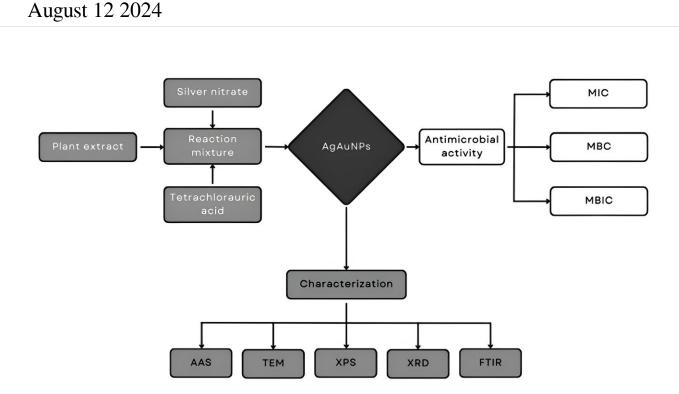
Flowchart summarizing the contents of the study, showing the bimetallic nanoparticle synthesis method and the subsequent physico-chemical characterization as well as antimicrobial activity experiments. Credit: University of Chemistry and Technology Prague
