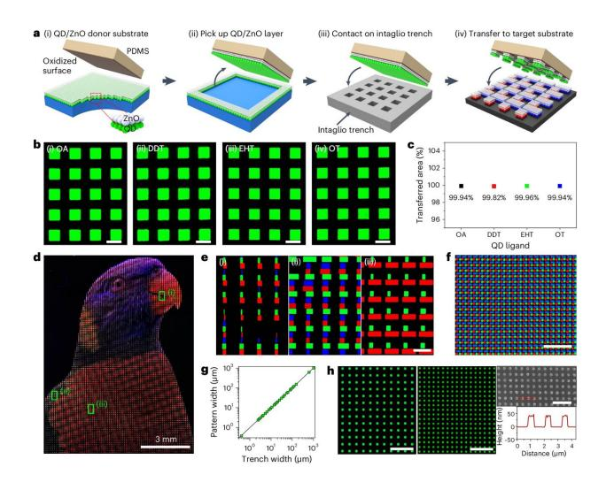
High-resolution intaglio transfer printing of QD/ZnO DL. Credit: *Nature Photonics* (2024). DOI: 10.1038/s41566-024-01496-x
