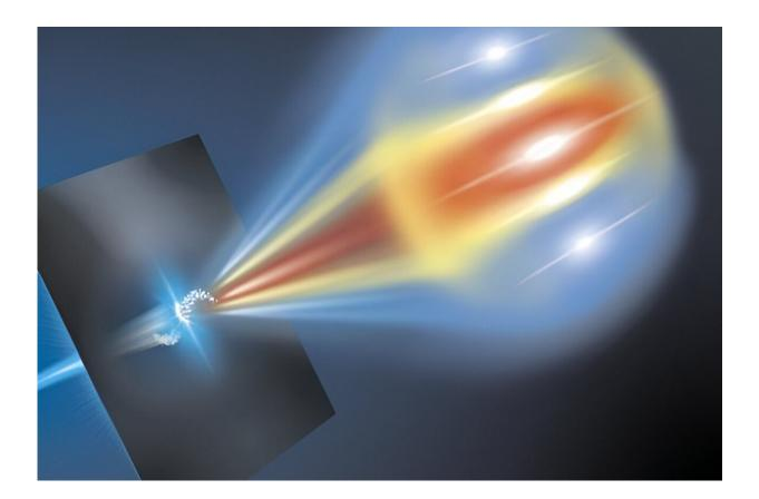
A structured beam of electron beamlets passes through a metallic foil from left to right creating coherent optical transition radiation. Credit: HZDR / Blaurock
