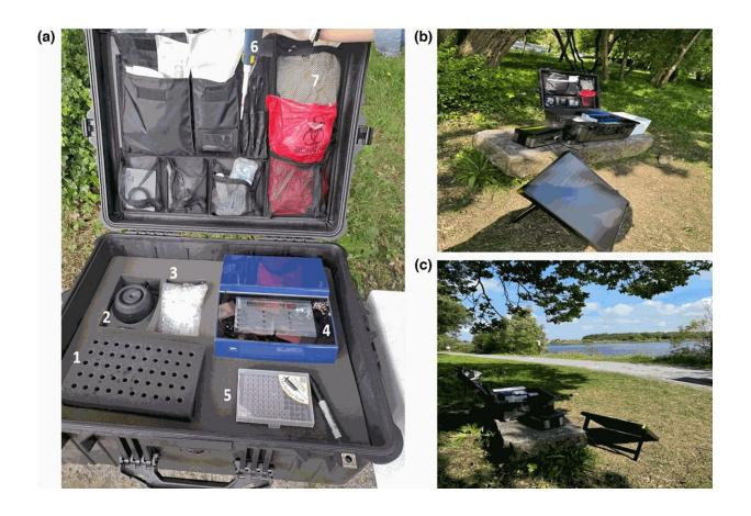
Portable diagnostics workstation. (a) Mobile workstation containing (1) microcentrifuge tubes rack, (2) vortex, (3) microcentrifuge tubes, (4) ESEQuant TS2 isothermal nucleic acid amplification instrument, (5) tips, (6) pipette and (7) laboratory consumables. (b, c) On-site application. Credit: *Microbiology* (2024). DOI: 10.1099/mic.0.001485
