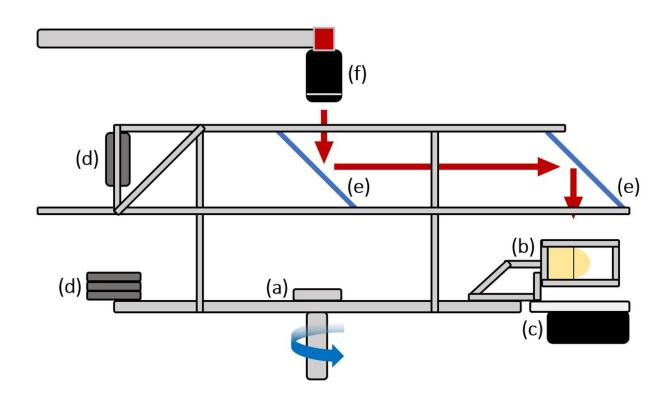
Schematic of the rotating wheel experimental facility, where (a) rotating disk, (b) test section, (c) LED light source, (d) counterweights, (e) mirrors, and (f) high-speed camera. Credit: Turbulent Mixing Laboratory/Lehigh University
