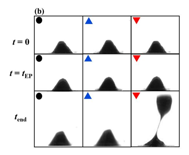
Snapshots of the perturbations with full elastic recovery and instability at t=0, @ t=EP threshold, and @ t=end of the experiment. Credit: Turbulent Mixing Laboratory/Lehigh University
