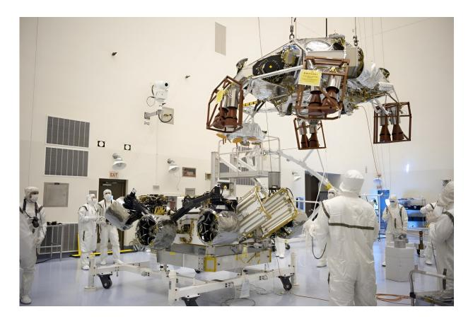
The rocket-powered descent stage that lowered NASA's Curiosity onto the Martian surface is guided over the rover by technicians at the agency's Kennedy Space Center in September 2011, two months before the mission's launch. Credit: NASA/Kim Shiflett
