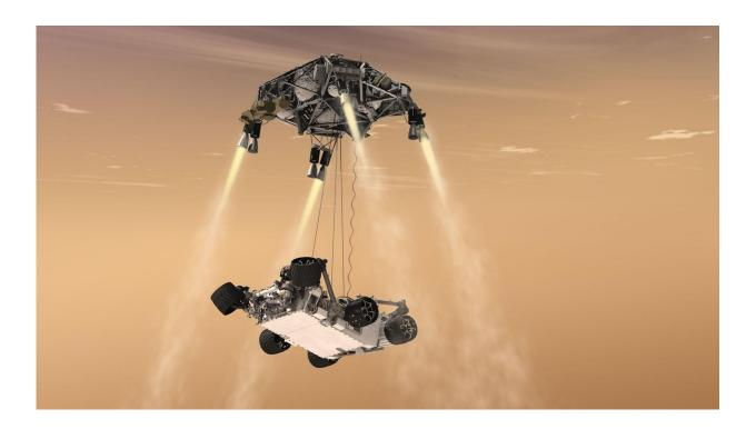
This artist's concept shows how NASA's Curiosity Mars rover was lowered to the planet's surface using the sky crane maneuver. Credit: NASA/JPL-Caltech
