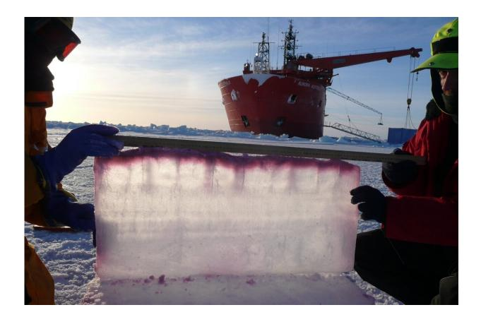
An upside-down sea ice slab showcasing brine channels that facilitate the drainage of liquid brine and support convection along the interface. Credit: Professor Ken Golden
