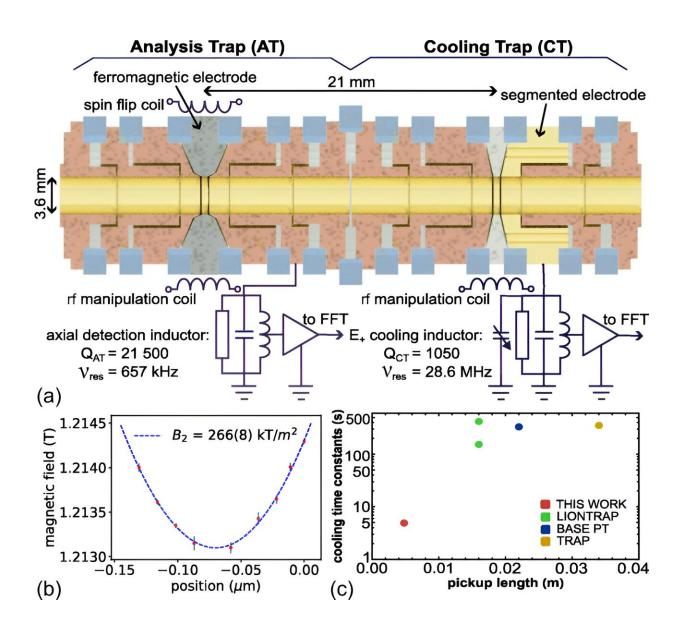
Double trap system, consisting of a cooling trap (CT) and an analysis trap (AT), with a superimposed magnetic bottle with a strength of  $\mathbb{R}_{AT}=266(8) \text{ kT/m}^2$ .
