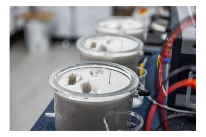
Samples of seawater-soaked sand in Rotta Loria's laboratory. The vertical, silver posts are electrodes. Credit: Northwestern University
