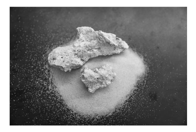
Sample of strengthened sand, treated with mild electricity, from the Rotta Loria lab. Credit: Northwestern University
