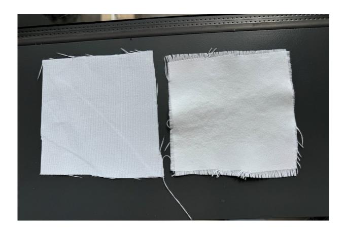
A chalk-based coating attaches to various commercially available textiles, including cotton and synthetic fiber, to create cooling fabrics, such as the treated synthetic material (right) that's brighter than the untreated fabric (left). Credit: Evan D. Patamia
