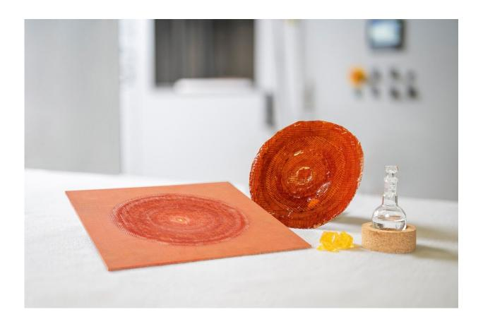
The moldable, recyclable polymer patch can take on any desired shape and size. Credit: Fraunhofer IFAM
