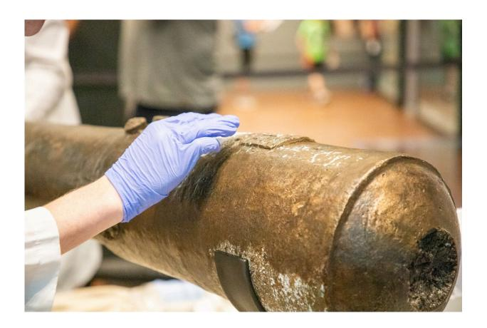
The Alamo cannon, post-acid solution treatment, which rapidly removed the carbonate blooms. Credit: Alamo Trust Inc.
