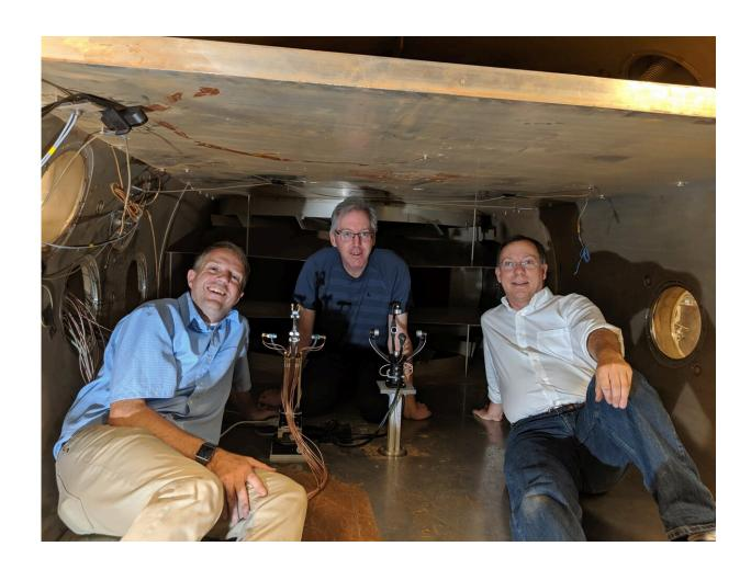
Authors Robert White (left), Ian Neeson (center) and Don Banfield (right) in the Mars Simulation Wind Tunnel at the University of Aarhus, Denmark in 2019, preparing to test early prototypes of the Mars sonic anemometer, visible in the center. The two prototypes were fabricated by Tufts University (left) and VN
