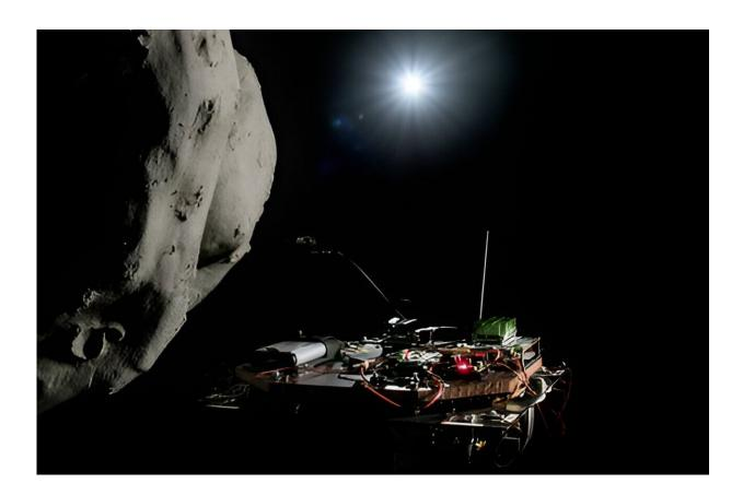
A close approach to a model comet in the Caltech Autonomous Robotics and Control Lab. This robotic spacecraft simulator mimics a space environment by floating on a low friction cushion of air and using air thrusters to maneuver. In newly published research, this robot is used by researchers at Caltech to demonstrate new capability for safe, real-time, autonomous fault estimation. Credit: Joshua Cho, Sorina Lupu, and James Ragan
