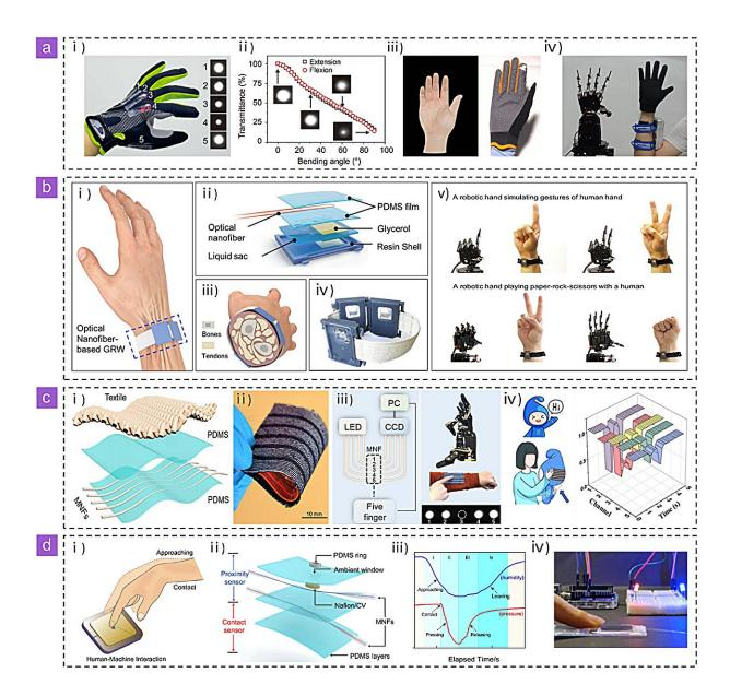
MNF tactile sensors for human machine interaction. Credit: OES
