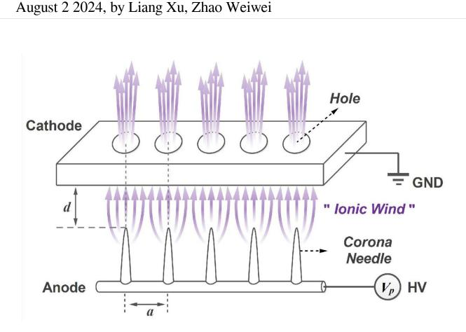
Schematic diagram of the EHD system structure of multi-needle. Credit: Liang Xu
