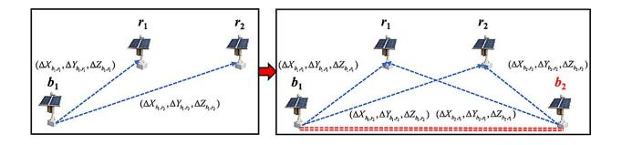
Deformation Monitoring Networks: Single-Base vs. Dual-Base Constraint. Credit: *Satellite Navigation* (2024). DOI: 10.1186/s43020-024-00148-3
