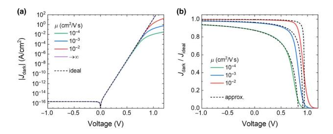
(a) Simulated dark current densities at different mobilities with 22 of 10 cm<sup>3</sup>/s. (b) Normalized dark current densities relative to the idealized expected dark current density in the limit of high mobilities. Credit: *PRX Energy* (2024). DOI: 10.1103/PRXEnergy.3.023008
