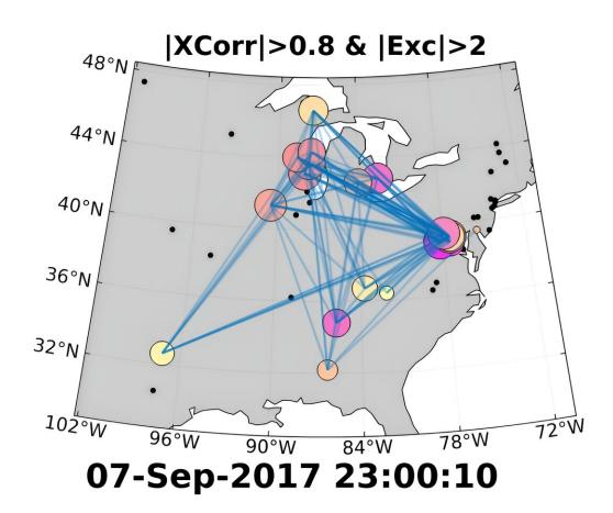
A snapshot of the geomagnetically induced current (GIC) network during an intense solar storm in September 2017. British Geological Survey. License type Attribution (CC BY 4.0). Credit: Royal Astronomical Society
