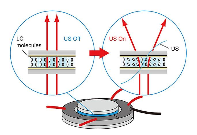
Schematics of the LC molecular orientation and the transmitted light in the absence (left) and in the presence (right) of the ultrasound excitation. Red and blue curves represent the light and the ultrasound vibration, respectively. Credit: Daisuke Koyama / Doshisha University
