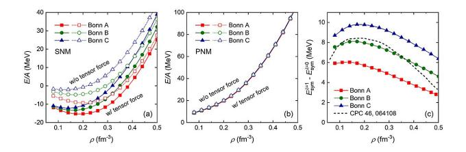
The binding energies per particle for (a) symmetric nuclear matter (SNM) and (b) pure neutron matter (PNM) calculated with (solid lines and full symbols) and without (dotted lines and empty symbols) tensor forces. (c) The symmetry energy difference obtained by performing the RBHF calculations with and without tensor force. Credit: Science China Press
