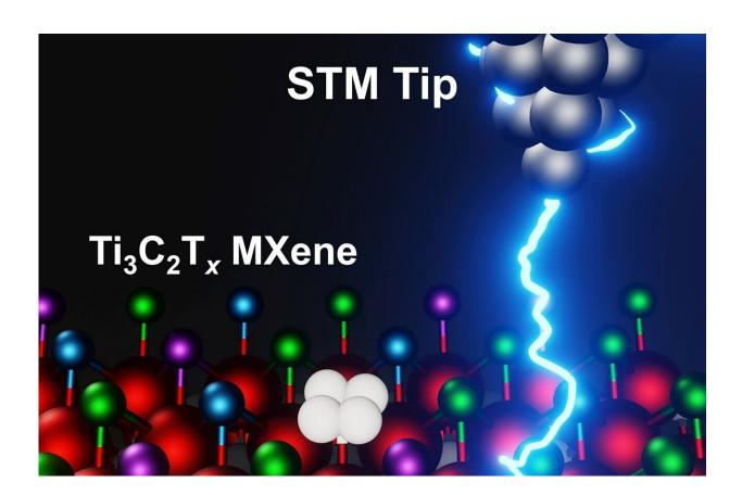
Using scanning tunneling microscopy, researchers at Drexel University and UCLA are providing the first atom-scale look at the surface of 2D MXene materials. The findings will help to tailor the unique materials for specific applications. Credit: Drexel University
