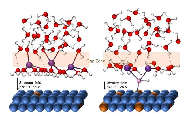
The mechanism of HOR catalyzed by Ni-W alloy. Credit: University of Science and Technology of China
