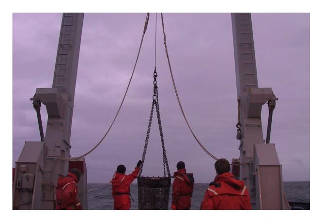
The stern of the research vessel, the R/V Knorr while at sea in 2004. The A-frame structure holds the giant metal and chain bucket which is lowered more than 10,000 feet below the ocean surface and dragged along the seafloor to collect geologic samples. Credit: Emily Van Ark
