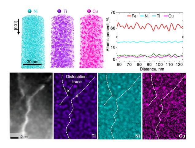
Analysis of spinodal decomposition and strengthening using nano-atomic-scale analysis. Credit: POSTECH
