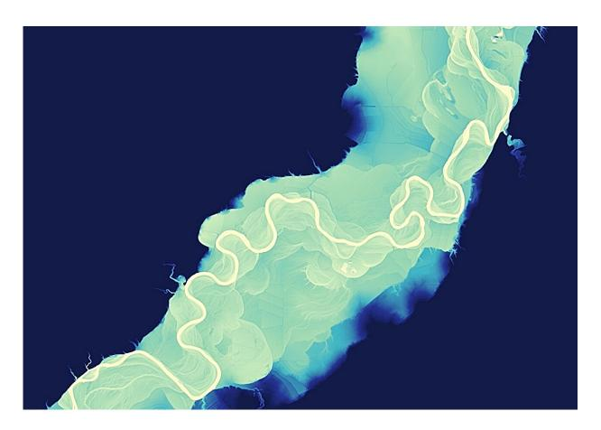
Relative Elevation Model of the floodplain of the Powder River, Montana. Example of high Overbank Hydrologic Variability (OHV) with prevalent chute cutoff. Credit: Riccardo Maitan
