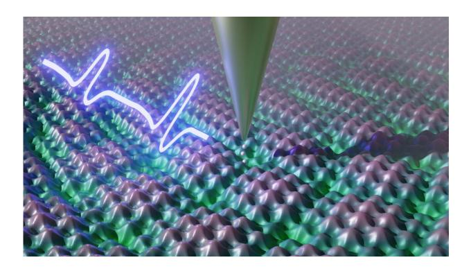
The imaging tip of the time-resolving scanning tunneling microscope captures the collective electron motion in materials through ultrafast terahertz pulses. Credit: Shaoxiang Sheng, University of Stuttgart (FMQ)
