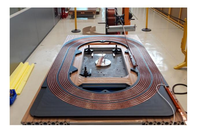
The coil of the prototype magnet is made up of superconducting magnesium diboride cables. Credit: CERN
