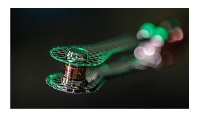
In inertial confinement fusion experiments, lasers at Lawrence Livermore National Laboratory's National Ignition Facility focus on a tiny fuel capsule suspended inside a cylindrical X-ray oven called a hohlraum. Credit: Jason Laurea, Lawrence Livermore National Laboratory
