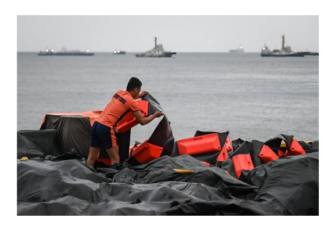
A coast guard staffer arranges an oil spill containment boom to be used in Manila Bay.
