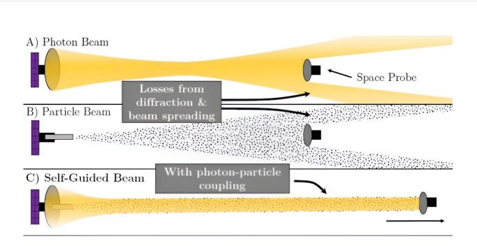
Depiction of the diffraction issues with particle a photon beams, and how a "selfguided" combined beam keeps providing pushing power even to probes that are far away. Credit: Limbach & Hara
