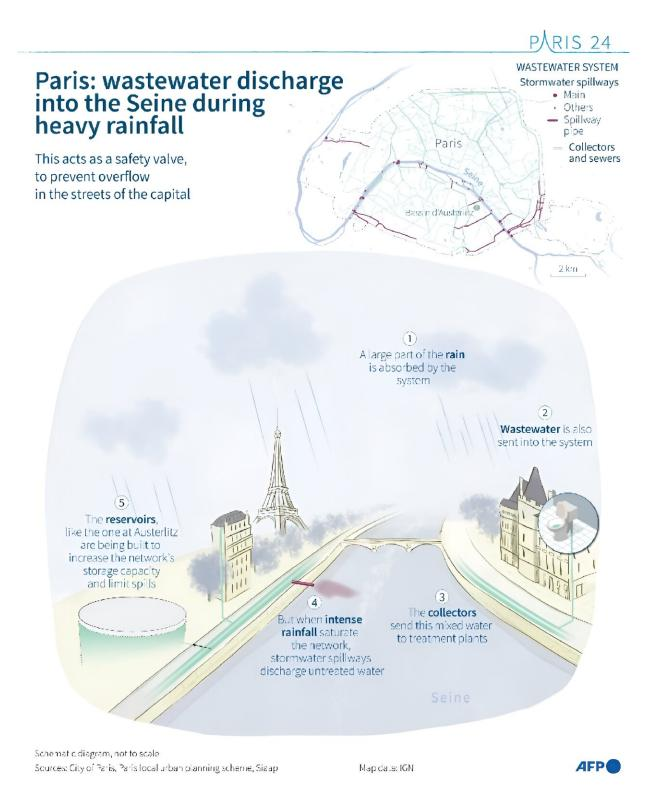
Diagram showing how untreated wastewater is discharged into the Seine during heavy rainfall in Paris.
