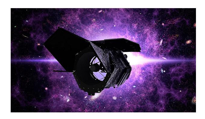
Artist's impression of the Nancy Grace Roman Space Telescope. The actively cooled primary mirror has a diameter of 2.4 metres. It is a copy of the primary mirror of the Hubble Space Telescope. The scientific objectives are to explore dark matter, dark energy and exoplanets. The Coronagraph Instrument (CGI), in whose development and construction the MPIA is involved, tests a new observation technique for the search and study of exoplanets. Credit: GSFC/SVS
