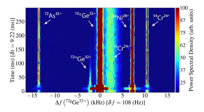
Time after injection ([2][2][2]=9.22 ms per time bin) versus revolution frequency ([2][2][2]=108 Hz per frequency bin) spectrogram of the sum of 102 single injections (setting 1) centered on <sup>72g</sup>Ge<sup>32+</sup> from 0 to 300 ms. The power spectral density of each ion species is proportional to their ion number. Credit: *Physical Review Letters* (2024). DOI: 10.1103/PhysRevLett.133.022502
