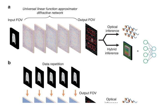
Different nonlinear encoding methods for diffractive optical processors using linear optical materials. Credit: *Light: Science & Applications* (2024). DOI: 10.1038/s41377-024-01529-8
