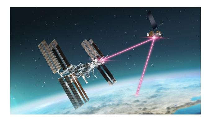
A graphic representation of a laser communications relay between the International Space Station, the Laser Communications Relay Demonstration spacecraft, and the Earth. Credit: NASA/Dave Ryan
