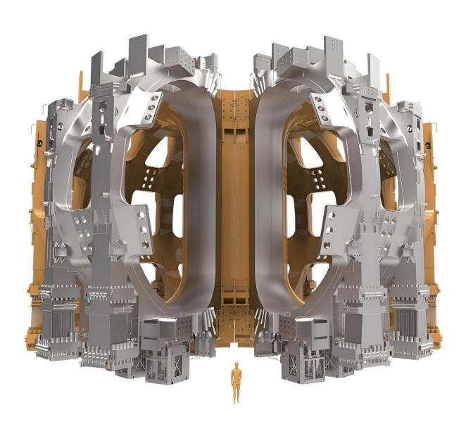
How the toroidal field coils fit around the tokamak vacuum vessel (including
